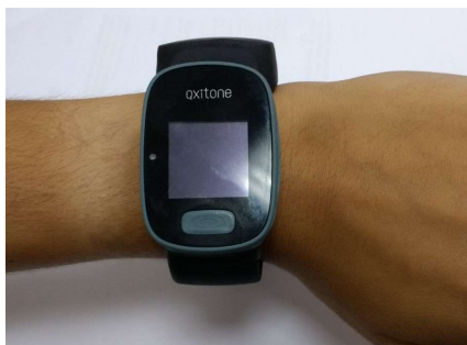
Correct placement of device, with the U-shaped part of device on top of the Ulna bone
