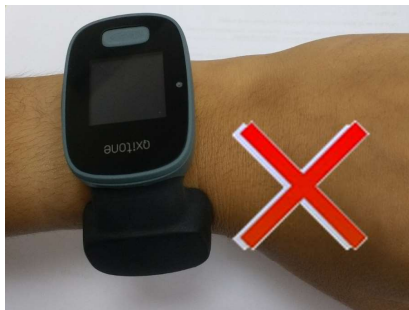
Incorrect – device upside down
